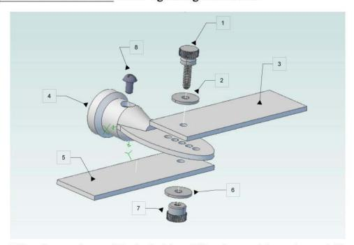
After placing paddling feet on decoy- Wonderduck's paddling feet work best when paddling foot is on outside foot attachment as it strikes the water. If paddling feet are not in correct position - do not remove feet - but slightly loosen nut on set screw - rotate feet - then retighten nut on screw. This feature will allow you to control the water motion depending on the position of the feet.
